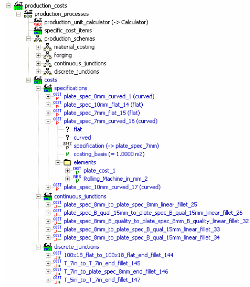
Fig. 13: a costing database generated from processes. The elements of each map to the individual processes which produced the cost definition
